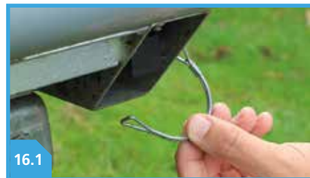
D-PIN SECURES BED SUPPORTS
