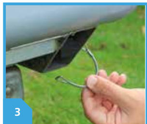
3. REMOVE THE D-PIN TO RELEASE LEG
