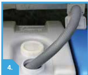
4. WASTE PIPE CONNECTION
