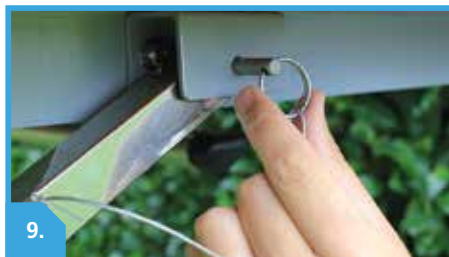
9. SECURE TOP OF LEG WITH PULL PIN TENT INFLATION
