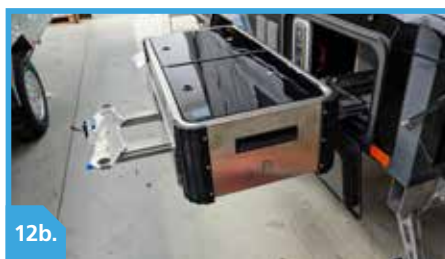
12b. LIFT AND ROTATE SLIDE-OUT HOB
