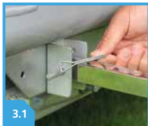
3.1 SECURE BASE OF LEG WITH D-PIN
